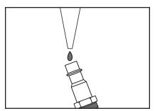
Figure 14. Lubricating sander via air inlet.
